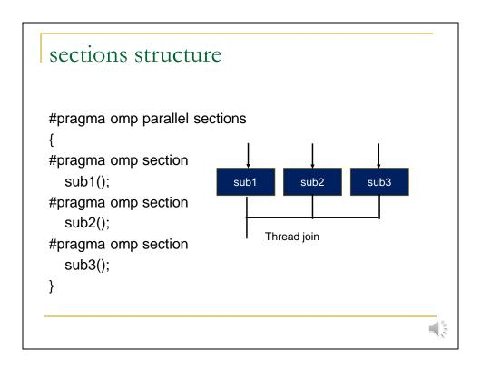
Forked threads can execute completely different program block. In this example, three subroutines are executed in parallel.
