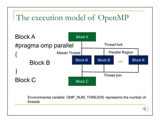
This is the execution mode of OpenMP, when the directive omp parallel is used, the block B in the program structure is forked and the threads are executed in parallel. After finished all threads, the join operation is executed.
