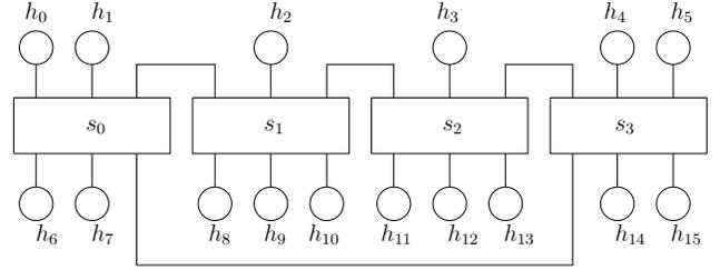
Fig. 1. An example of a host-switch graph ( $n = 16, m = 4, r = 6$ ). A circle and a rectangle represent a host and a switch, respectively.
