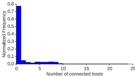
Fig. 8. Host distribution of a host-switch graph with unused switches  $((n, m, r) = (1024, 1024, 24))$ .
