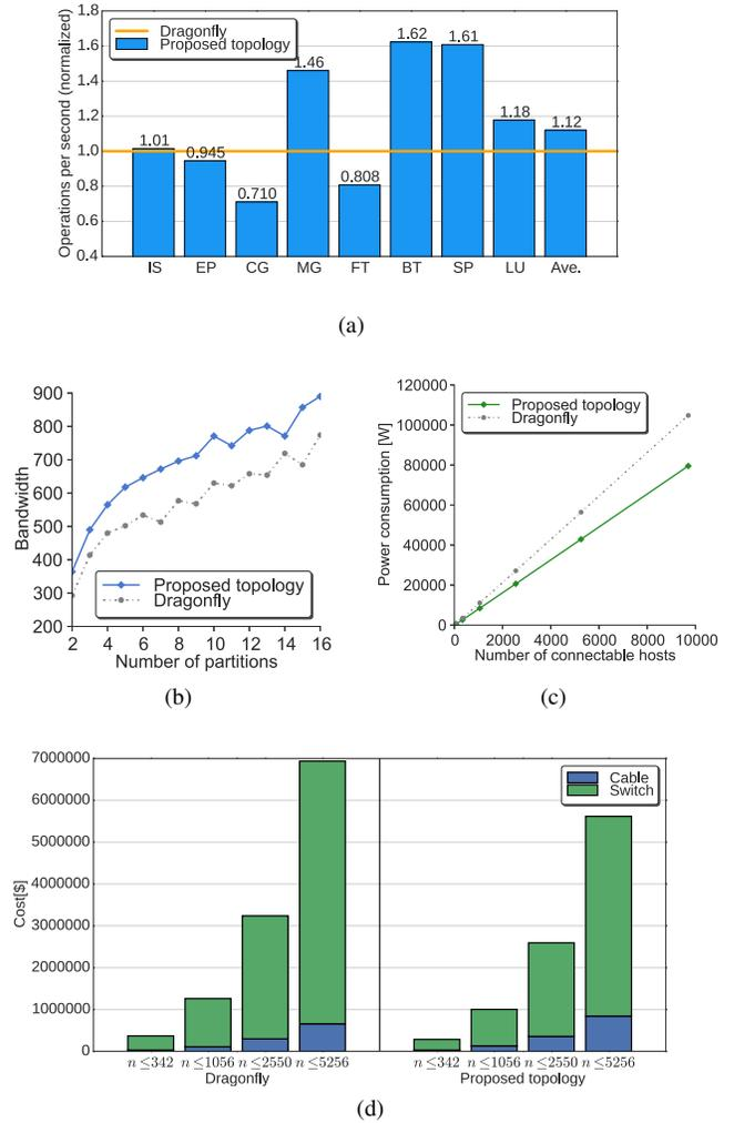
Fig. 10. Results of comparisons between dragonfly and proposed topology: (a) Performance; (b) Bandwidth; (c) Power consumption; (d) Cost breakdown.
