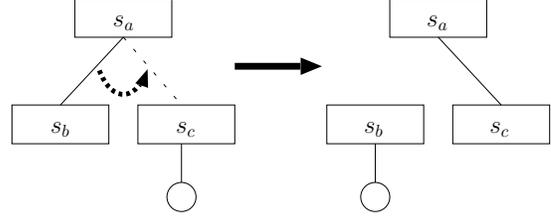
Fig. 3. Swing operation denoted as  $\text{swing}(s_a, s_b, s_c)$ .
