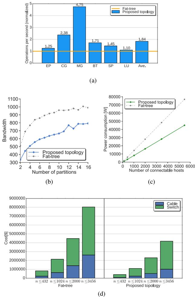
Fig. 11. Results of comparisons between fat-tree and proposed topology: (a) Performance; (b) Bandwidth; (c) Power consumption; (d) Cost breakdown.
